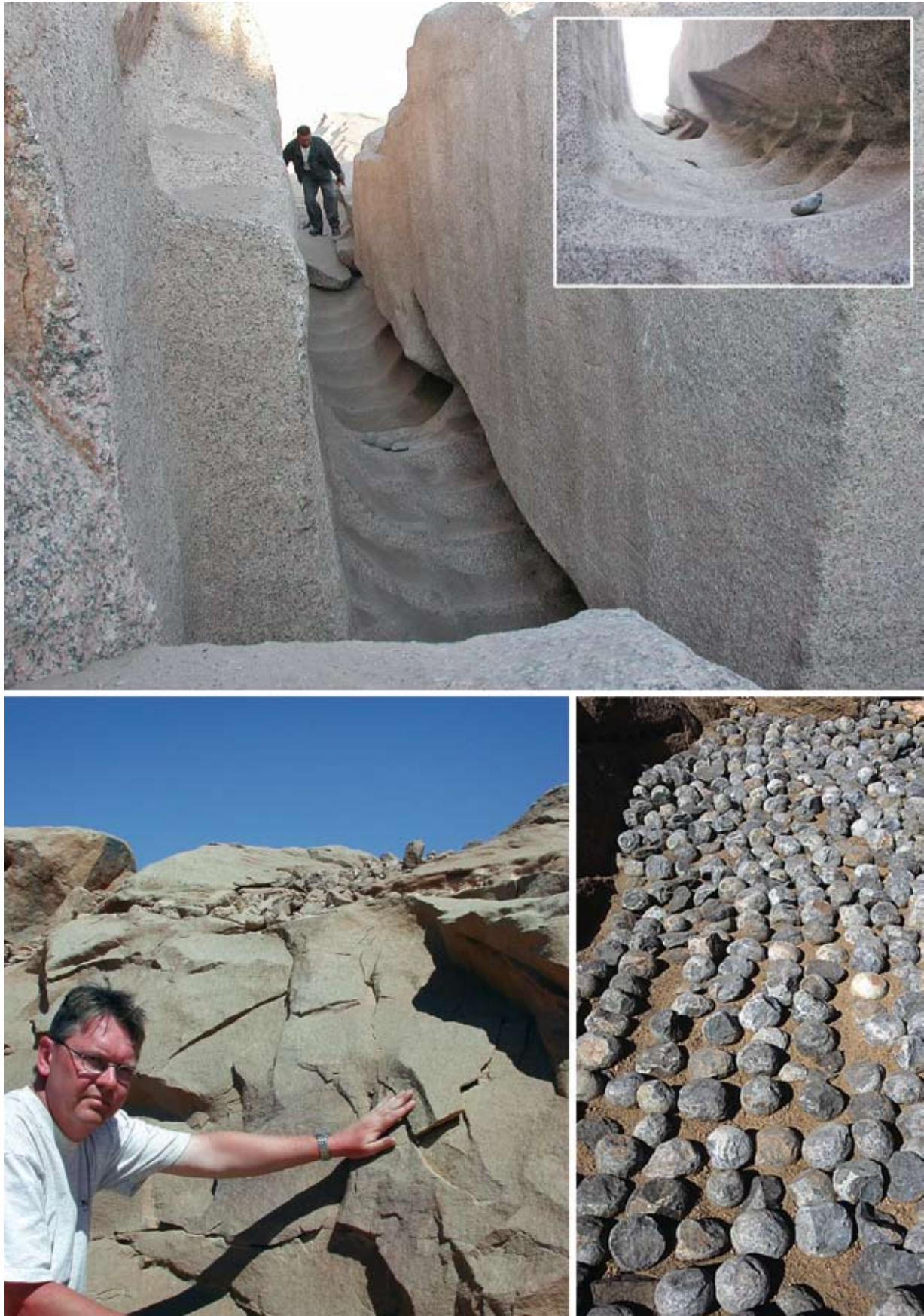
Figure 16. New Kingdom hardstone quarrying technology at Aswan. Top and upper insert: trenches cut in granite for a colossal statue in the Unfinished Obelisk Quarry at Aswan (part of H6) using dolerite pounders like those shown at bottom right. Bottom left: cracked quarry face produced by fire setting in the silicified sandstone quarry on Gebel Gulab (H5) near Aswan. Geologist Tom Heldal pictured. Photos by Per Storemyr except the bottom right one, which is by James Harrell.
